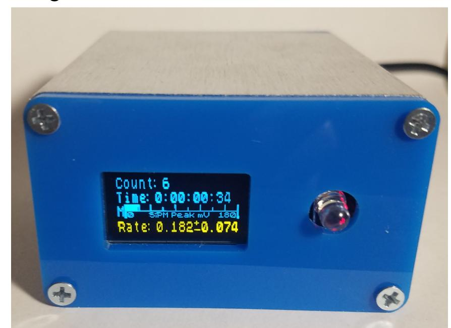
The OLED output display shows the total number of muon counts on the first line, the elapsed time on the second line, the detected SiPM voltage on the third line, and the rate of muons per second on the bottom line.
