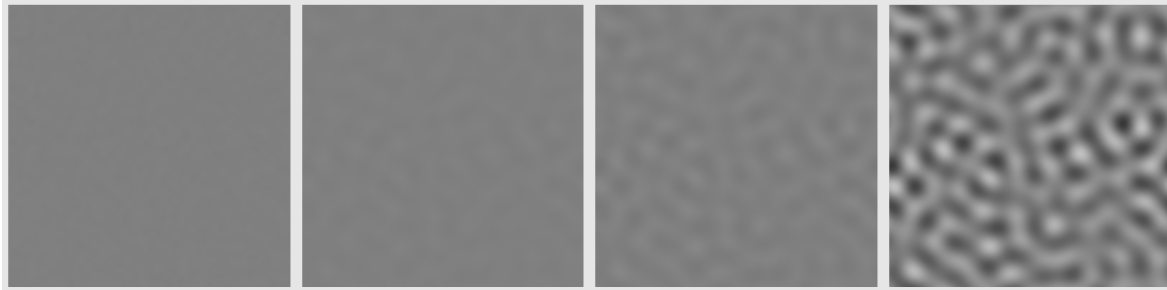
Figure 13.17: Simulation of the Turing pattern formation model with (a, b, c, d) = (1, -1, 2, -1.5) and (D_u, D_v) = (10^{-4}, 6 \times 10^{-4}) . Densities of u are plotted in grayscale (darker = greater). Time flows from left to right.
