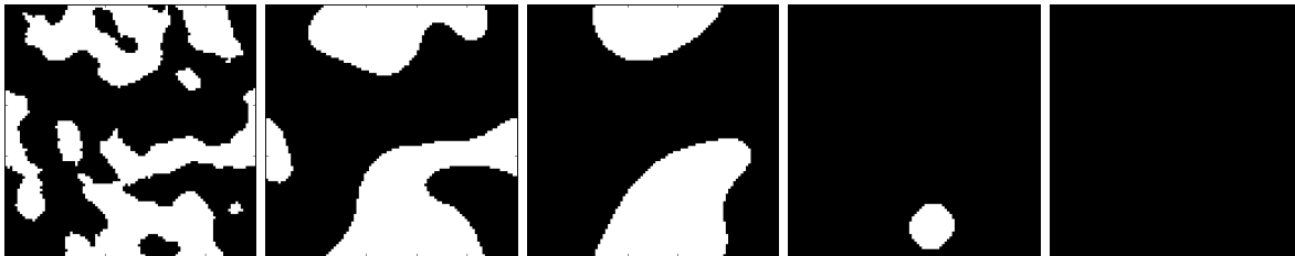
Figure 11.8: Coarsening behavior observed in a binary CA with the majority rule in a 100 \times 100 2-D spatial grid with periodic boundary conditions. The radius of the neighborhoods was set to 5. Time flows from left to right.
