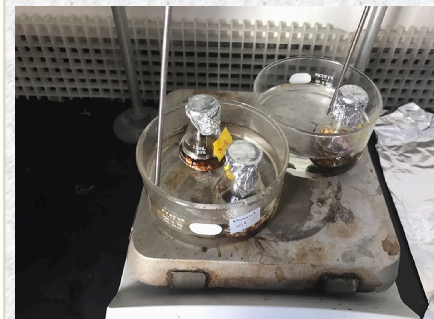
Figure 3. Acid Hydrolysis of Ground Alfalfa Hay and Ionic Liquid
