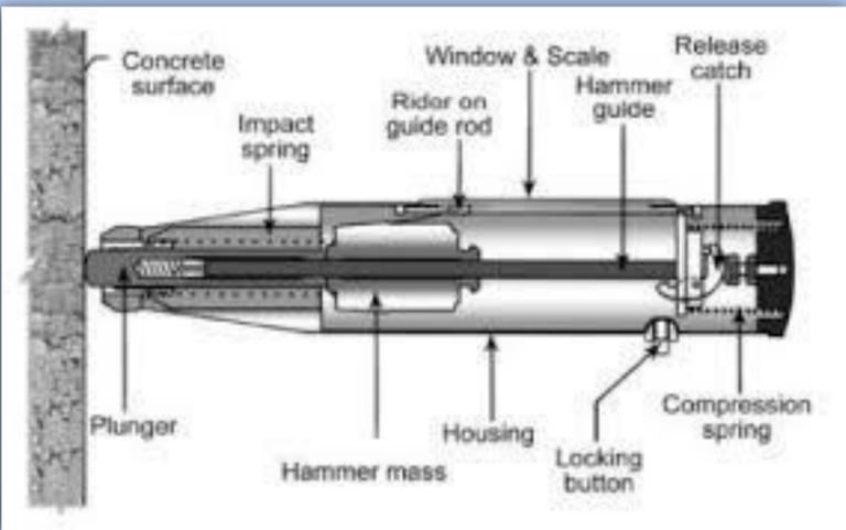
Figure 1: Cross sectional diagram of a Schmidt Hammer (From Jude Aruna Gayan via LinkedIn SlideShare)
