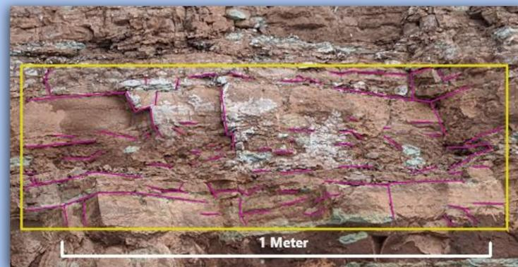
Figure 3: The same outcrop as shown in figure 2 with study area and fracture lines (in purple) overlain in Adobe Illustrator
