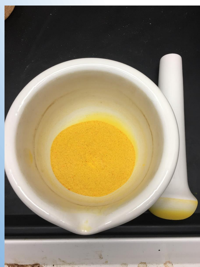
1 Grind (\text{NH}_4)_2\text{Cr}_2\text{O}_7 (orange) and washed sand to produce yellow mixture for 15 min
