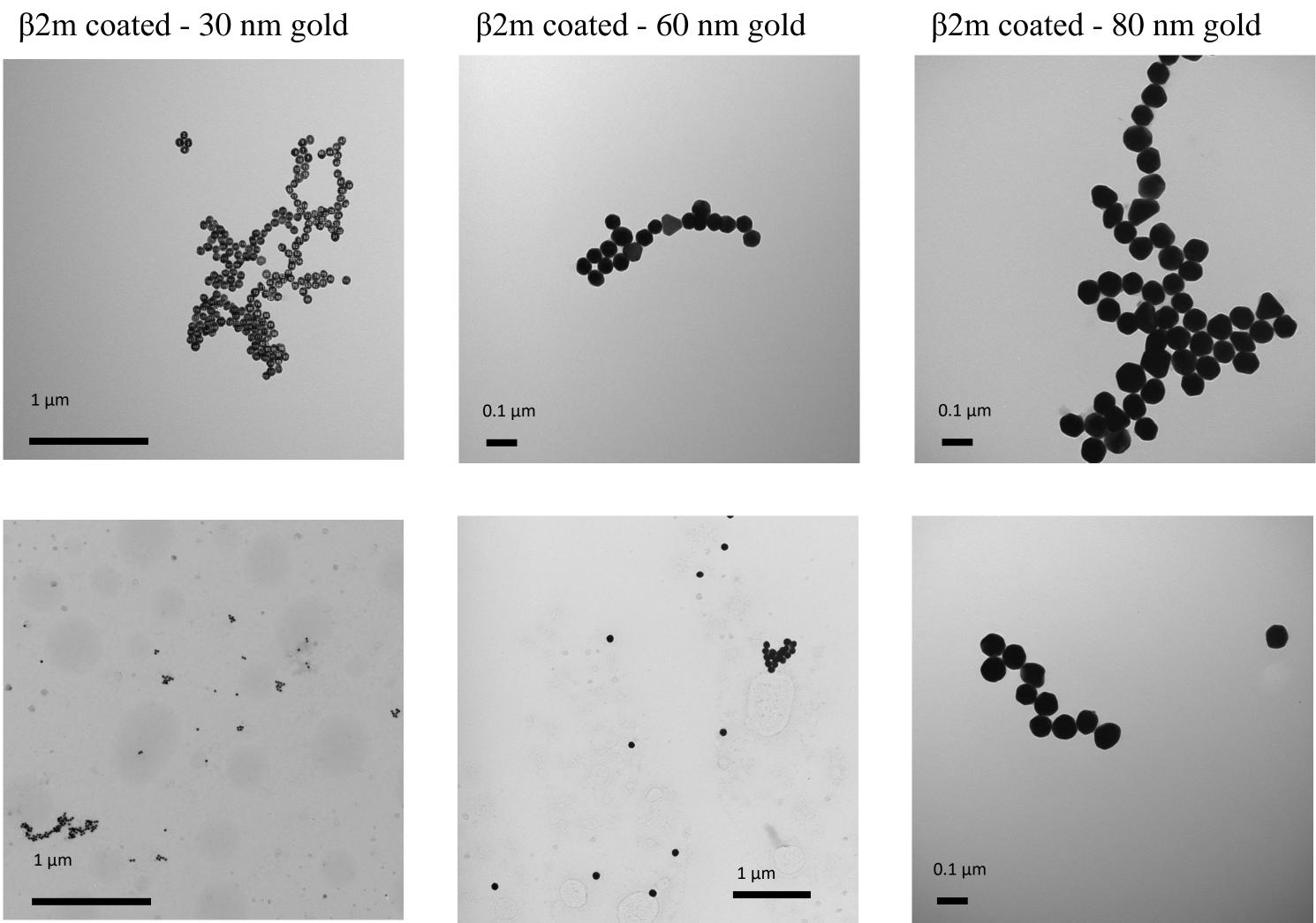
In certain aggregates, especially pH 4, we noticed spacing between adjacent gold nanoparticles. The space represents the region where peptide –peptide networking are taking place. Due to the limit in resolution by TEM, the peptide networking is not resolved. However, this spacing provides the best information of the dimension of the peptides to form networking at the interfacial environment.
