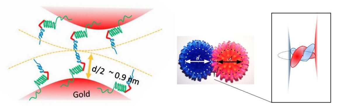
This study extracted that the distance between two adjacent gold nanoparticle is approximately 2 nm no matter the size of the gold colloid varies. On-going another project of our group disclosed that the orientation of the peptide is a "spiking - out". Considering that the dimension of longer axis is c.a. 9.2 nm, two peptides must face by "entangling" each other resulting in the distance between gold surface to be around 2 nm.
