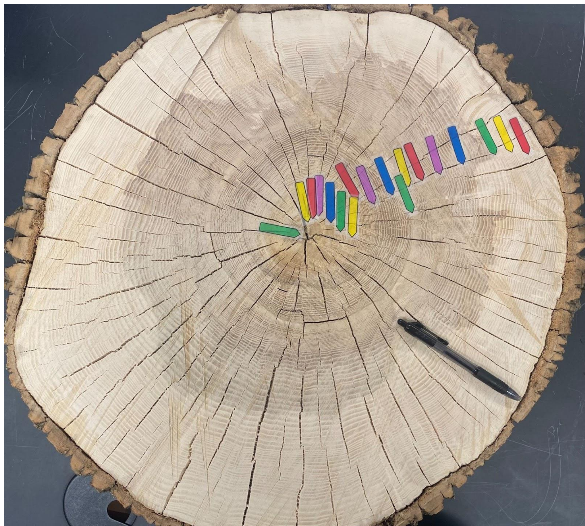
Figure 7: Ash tree taken from same Geneseo region as the other four samples. Tree is approximately 185 years old with ring thickness varying from 0.05mm to 6mm. Every 10 years is marked for reference while students are comparing and analyzing stresses of all five rings as well as adding historical dates. Pen for scale.
