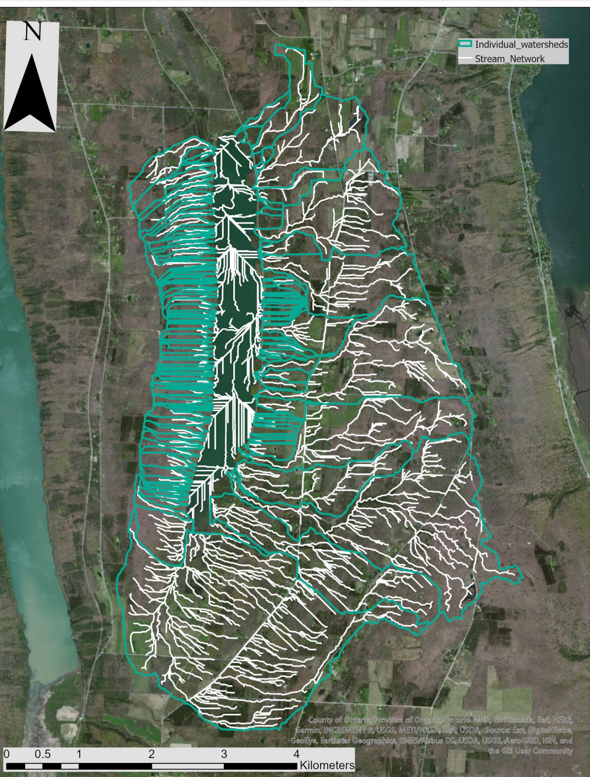
Figure 4. Stream networks and individual watersheds from flow accumulation grid and pour points
