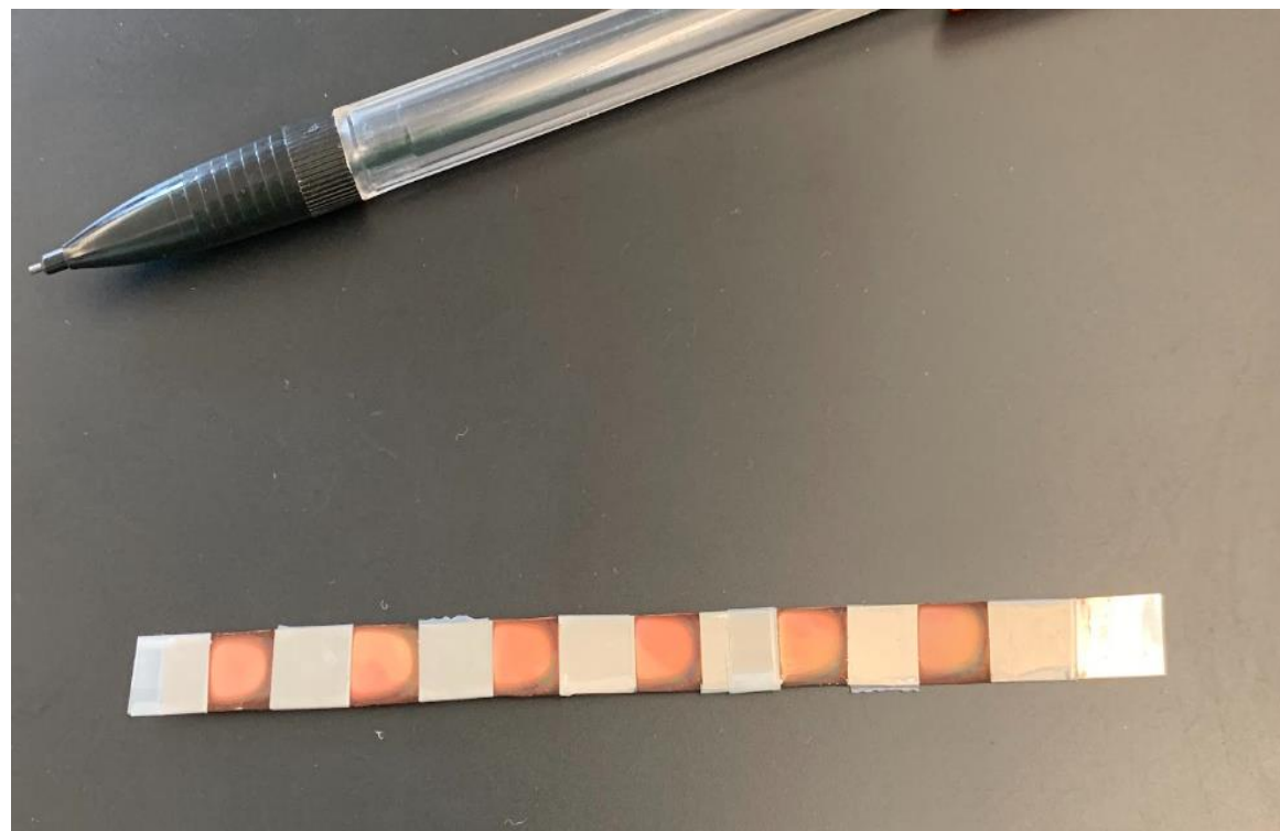
Left: Emma Parker and Kayla Andersen preparing a Cu coated W ribbon target in the SUNY Geneseo Chemistry laboratory. Right: A ribbon of tungsten with 1 micron thick sections of copper coating produced via electroplating.
