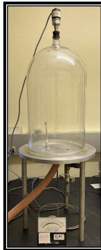
Thermocouple pressure gauge
