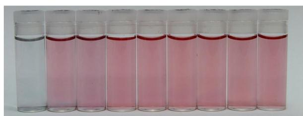
Left: A series of samples of sol-gel showing the pH dependence of the color. The left-most sample is pH 2 and the right-most sample is pH 10.
