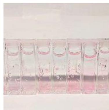
Left: A series of samples of sol-gel all with added HCl on top. No dispersion took place several hours of waiting.
