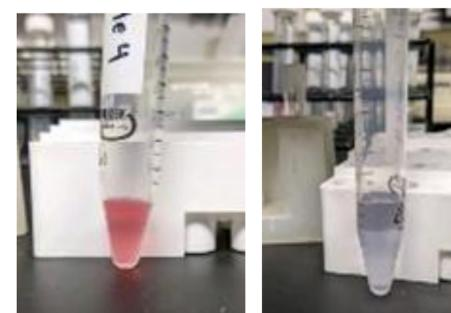
Right: Image of our sol-gel before and after the addition of HCl prior to the setting of the gel; can clearly see the color change.
