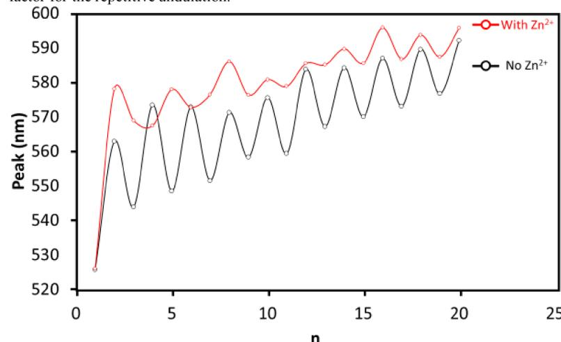
**Figure 4:** The results of the pH hop experiment with Zn<sup>2+</sup> ions and a control solution illustrates that the Zn<sup>2+</sup> solution with A $\beta$ (1-40) and the gold nanoparticles exhibits a decreased amplitude between acid and base peaks and the inability to return to a lower peak in acidic conditions. The peaks are also out of phase with Zn<sup>2+</sup> compared to no Zn<sup>2+</sup>.
