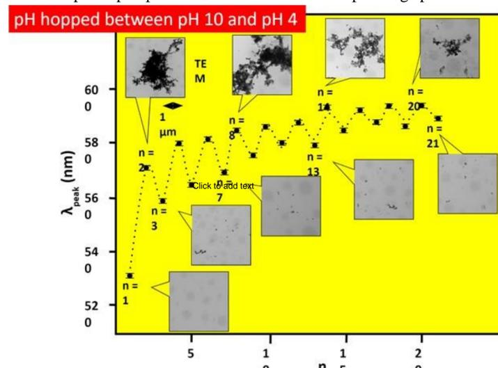
**Figure 3:** TEM image of A $\beta$ (1-40)-coated Au-20 nm at different operation numbers.
