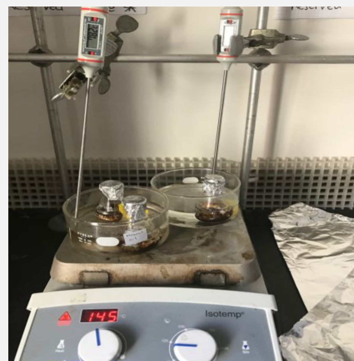
Figure 2. Samples are heated in a mineral oil bath for 3,6, or 9 hours at 80 degrees Celsius. A magnetic stirrer is added to completely mix the mixture
