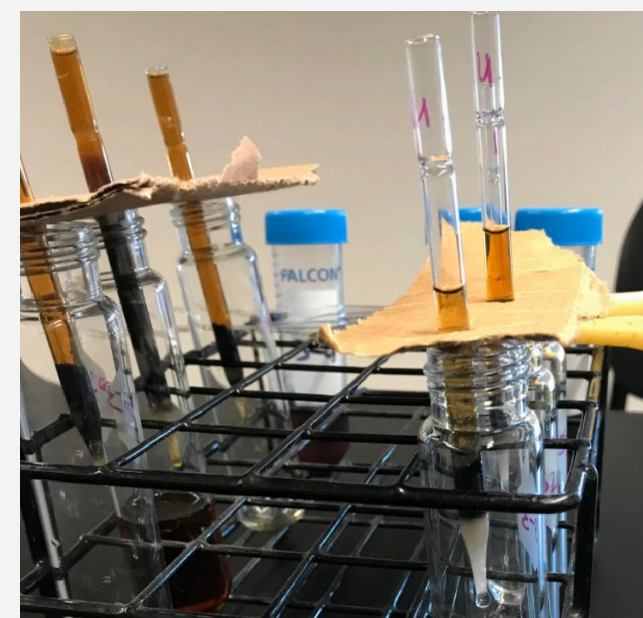
Figure 3. Centrifuged samples are subjected to a filtration system consisting of glass fibers, sand, and charcoal in a short-necked pipette. Solutions are filtered until clear.
