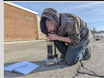
Fig. 4. A dial is turned in order to center the beam (null-position). Depending on which direction and how much the dial is turned, a gravitational anomaly value is then recorded. (Burger, 1992)
