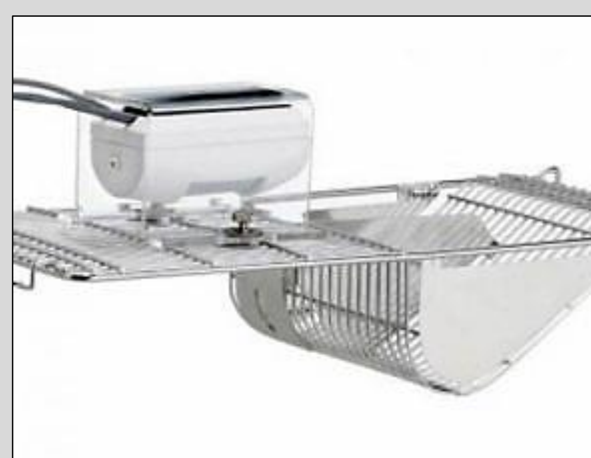
Figure 5. Pictured is the VitalView cage top monitor fastened on top of a typical rat cage topper.
