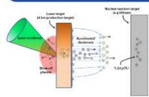
A light ion beam (e.g., deuterons) is accelerated from the rear side of a laser target illuminated with an ultra-intense laser (MTW or OMEGA). The light ion beam then strikes a nuclear reaction target (e.g., lithium) and initiates nuclear reactions. By counting the activity of the reaction products, the nuclear reaction cross section can be determined.
